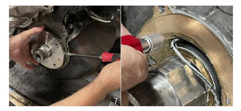
9. Install pump and harmonic balancer and start engine. Check for leaks.
